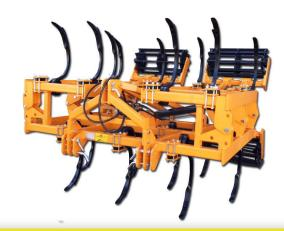
Frame clearance of 700mm. allows mixing of soil and its correct aeration.
